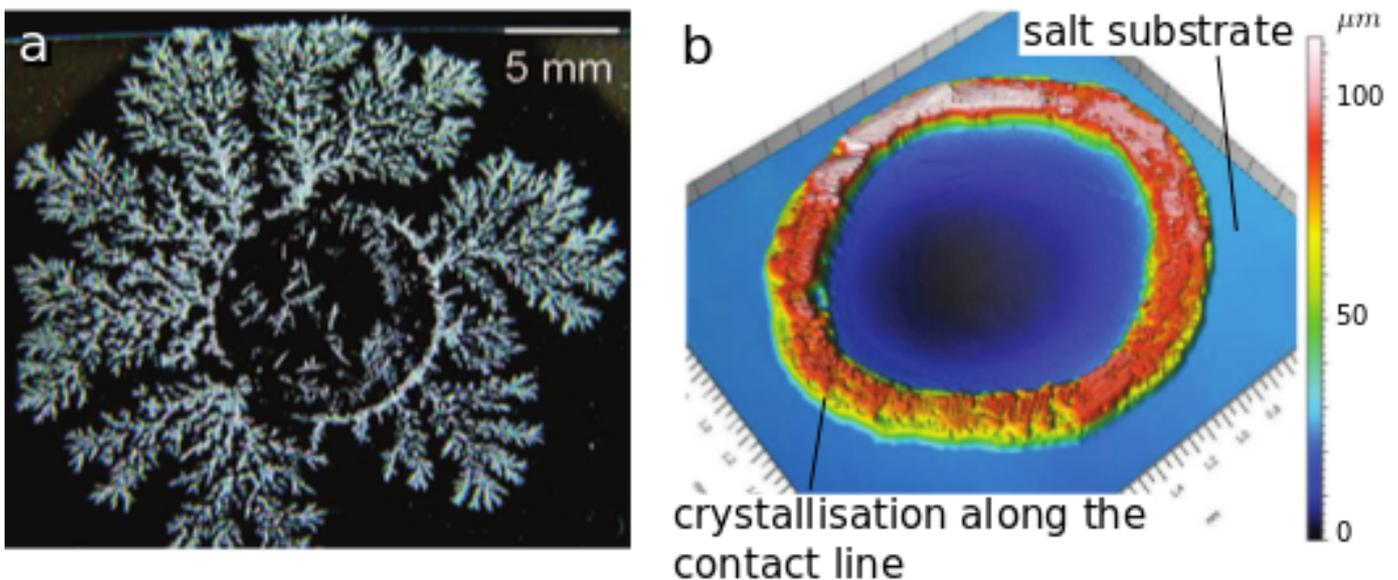
**Figure 1 :** a) The evaporation of a droplet of water charged in salt leads to a specific pattern (Shahidzadeh et al. 2008). b) The evaporation of a droplet of pure water on a salt substrate leads to the excavation of the substrate at the center of the droplet and the formation of a seam along the contact line (Mailleur 2016).
